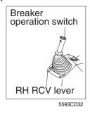
(1) On pressing this switch, the breaker operates only when the breaker selection switch on the switch panel is selected.
