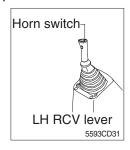
(1) This switch is at the top of left side control lever. On pressing, the horn sounds.
