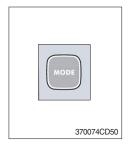
(1) Operating this switch, it beeps and displays symbol of each mode in order. (Vent → Vent/Foot → Foot → Foot/Def → Vent)
